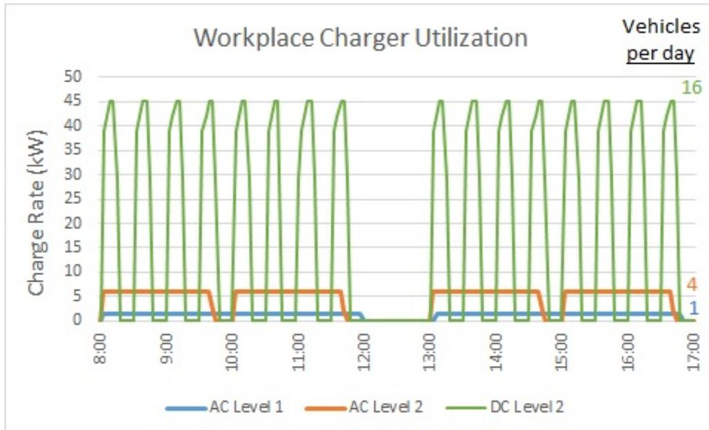
**Figure 5. Workplace Charger Operating Profile**
