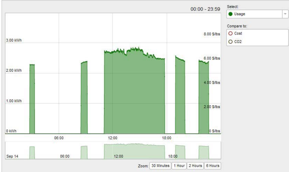
Figure 129. Site 40 condenser Stage 2 only operation
