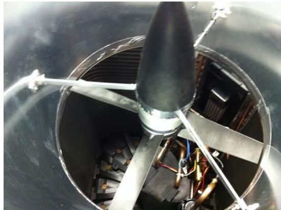
Figure 8. 40-degree pitch propeller with 9-degree divergent diffuser and conical center after body
