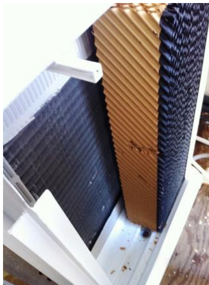
Figure 12. Showing the 6” evaporative media pads being installed in the water collection trough of the Phase II prototype
