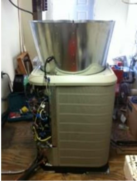
Figure 7. Nine-degree divergent diffuser under test
