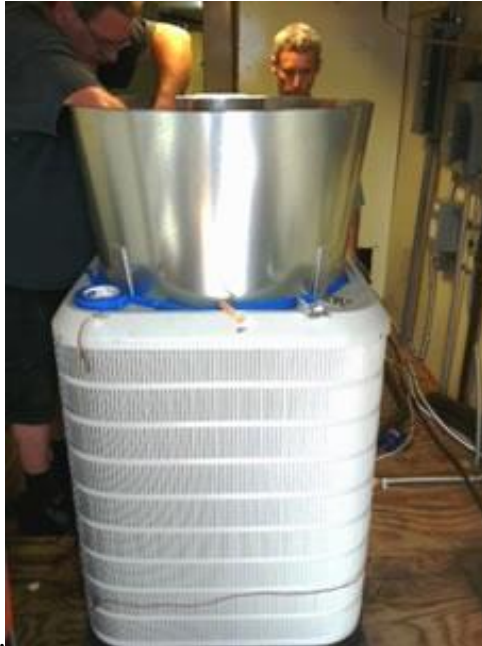
Figure 6. Fabrication of 7-degree divergent diffuser
