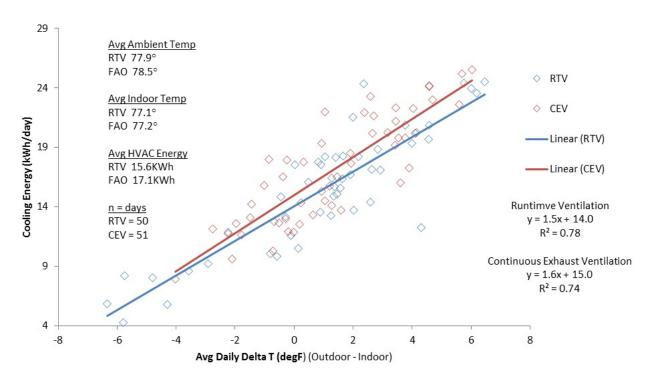
Figure 4. HVAC energy use as a function of differences in indoor and outdoor temperatures.
