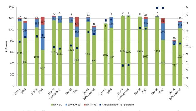
Figure 2. Distribution of hours at various % RH ranges, broken into runtime vent (left bar) and continuous exhaust (right bar) periods, each corresponding to the left axis. Numeric data labels correspond to hours, black squares correspond to average indoor temperature (on the right axis). Sites 3 and 5 always operate with continuous exhaust, and sites 7 and 10 always operate with runtime vent.
