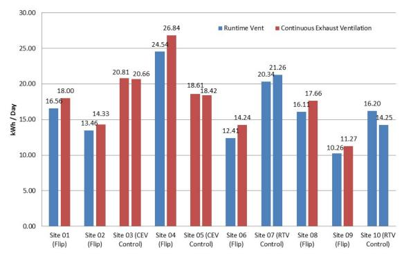
Figure 3. Average HVAC energy use per day, broken into runtime vent (left bar) and continuous exhaust (right bar) periods. Sites 3 and 5 always operate with continuous exhaust, and sites 7 and 10 always operate with runtime vent.
