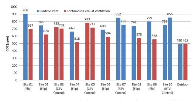
Figure 6. Daily average CO<sub>2</sub> concentration, broken into runtime vent (left bar) and continuous exhaust (right bar) periods. Sites 3 and 5 always operate with continuous exhaust, and sites 7 and 10 always operate with runtime vent.
