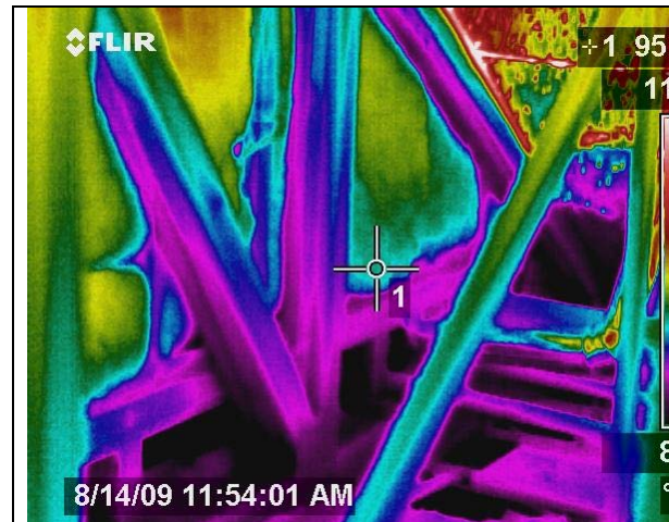
Figure 7 IR view inside the attic shows cool temperatures in the floor space and cooled surfaces low in attic. (Withers)
