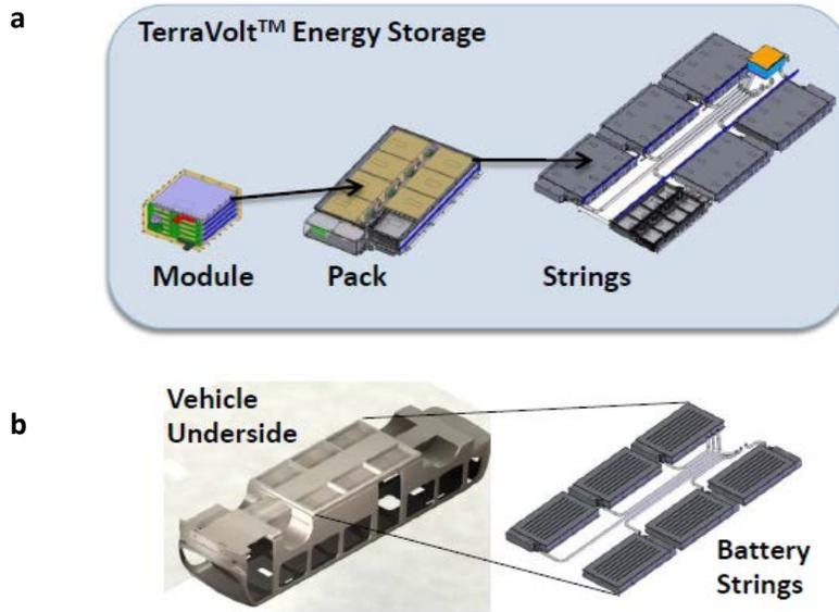
**Figure 3. The energy storage system of a Proterra electric bus.**
