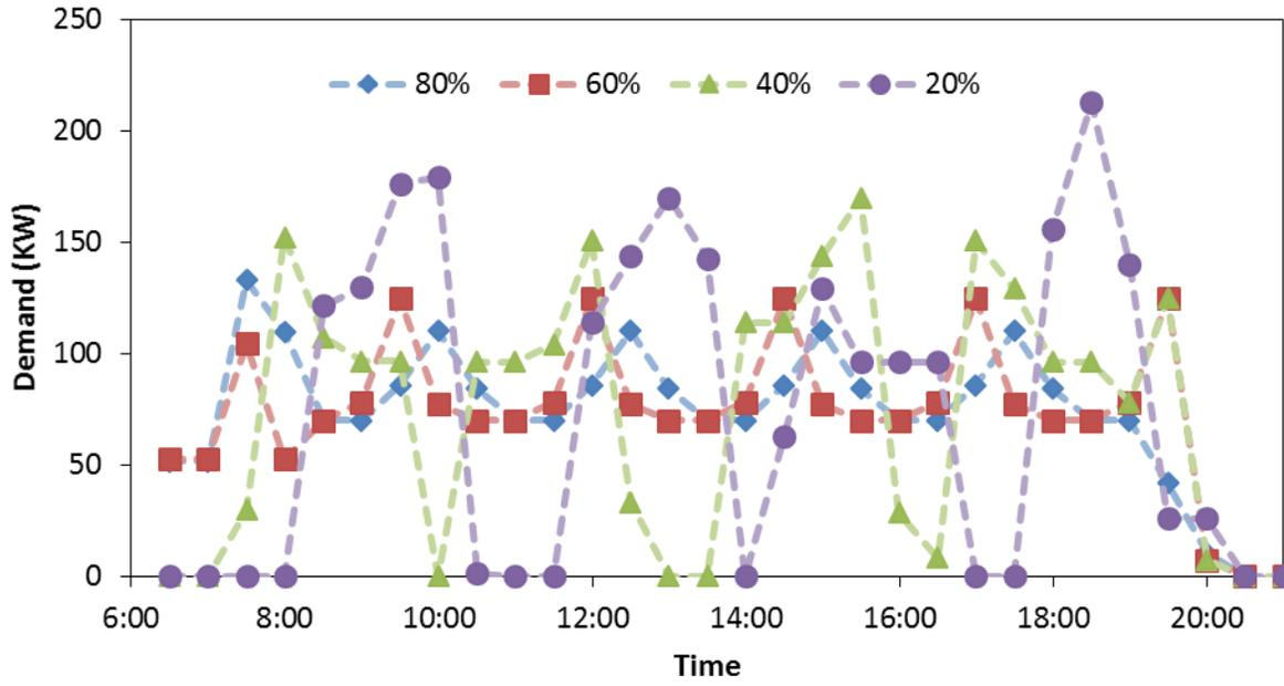
Figure 13. Daily demand profiles using different charging thresholds
