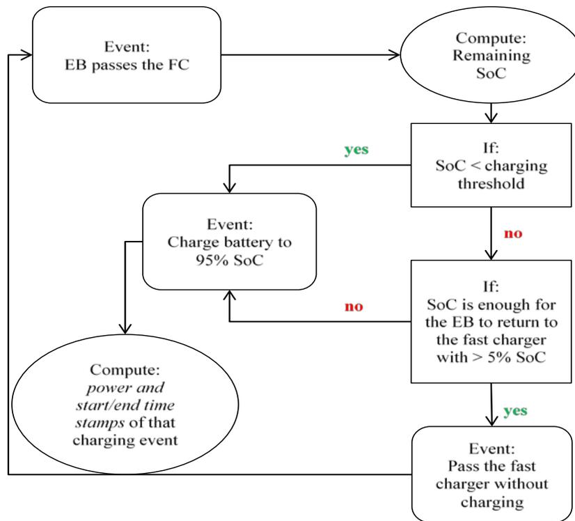
**Figure 11. Schematic representation of the charging model**
