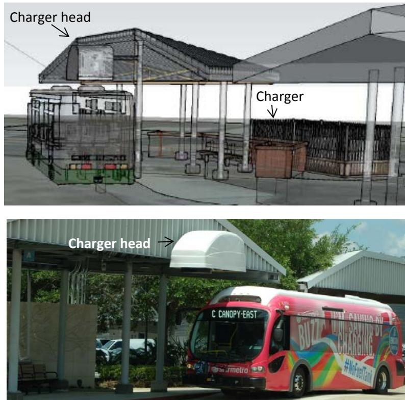
**Figure 5. The model and actual picture of the FastFill™ charger and the charger head.**
