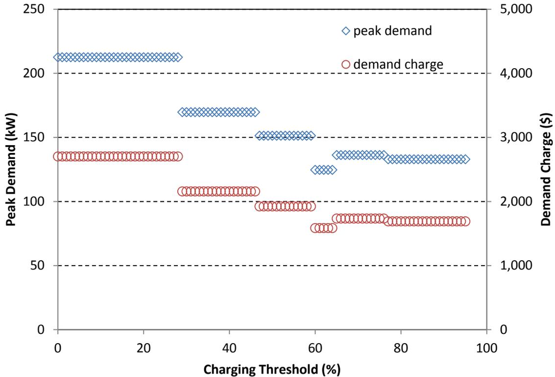
**Figure 12. Peak demand and demand charge at different charging thresholds for 5 EBs**
