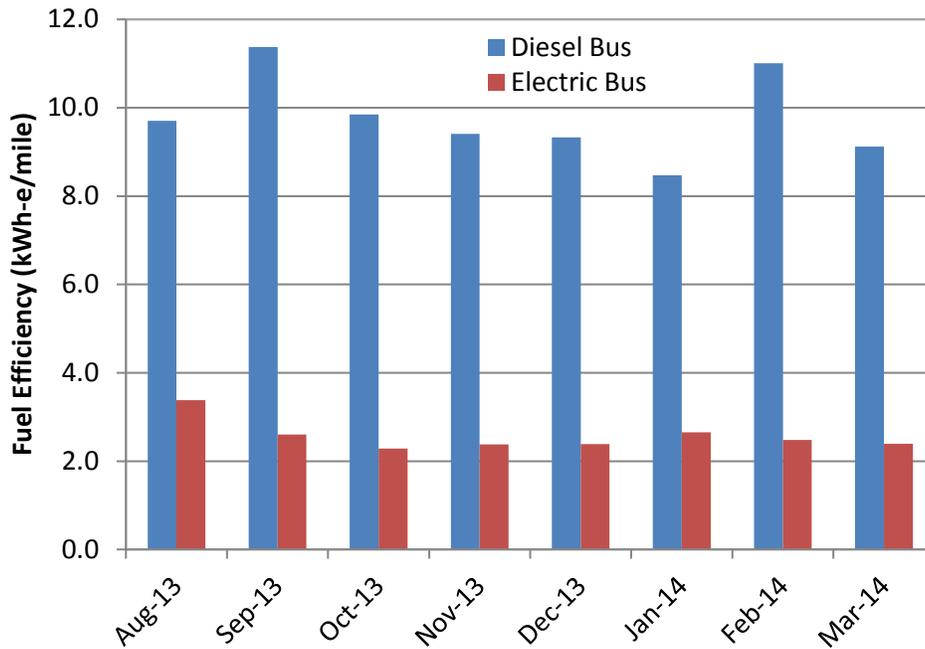
**Figure 7. Fuel efficiency comparison of EBs and DBs from August 2013 to March 2014.**
