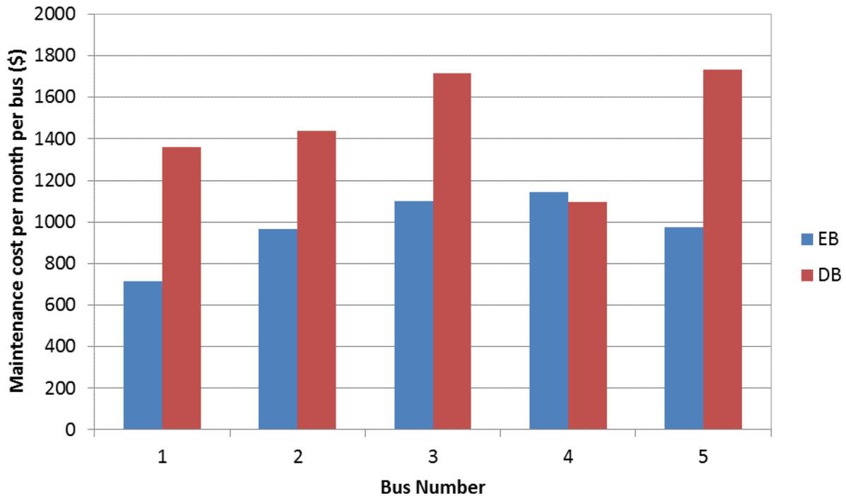
**Figure 10. Maintenance cost comparison between EBs and DBs from Aug 2013 to Mar 2014**
