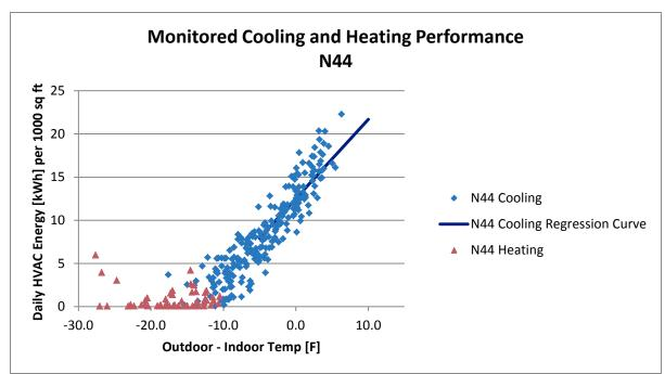
Figure A-41 Monitored Cooling and Heating Performance, N44
