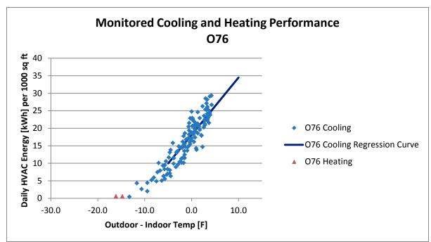
Figure A-205 Monitored Cooling and Heating Performance, O76
