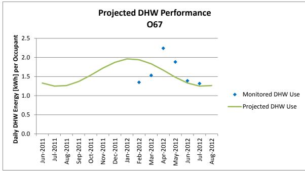
Figure A-201 Projected DHW Performance, O67
