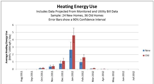
Figure 7-3. Heating Energy Use by Month, Utilizing Monitored and Utility Bill Data Projections.
