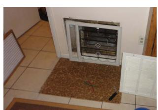
Figure 4-31. An airflow measuring plate sensor that measured air conditioner airflow is seen at the return intake. This was placed at the air handler inside the filter access slot when possible.
