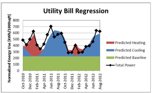
Figure 5-5. Results of multiple regression analysis on utility bill data using cooling degree days and heating degree days.
