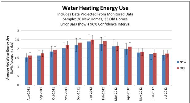
Figure ES-3. Monthly Hot Water Energy Use Results, Utilizing Monitored and Utility Bill Data Projections.
