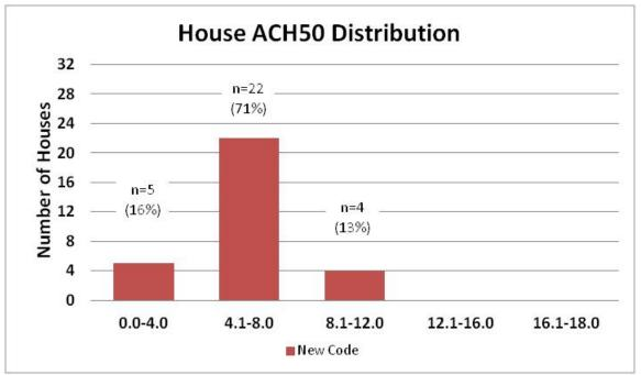
Figure 7-31. Normalized house leakage distribution for the new code group (n=31).
