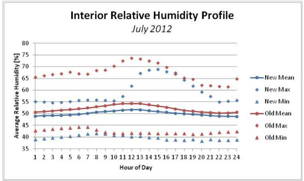
Figure 7-29. Interior Relative Humidity Profile, July 2012.
