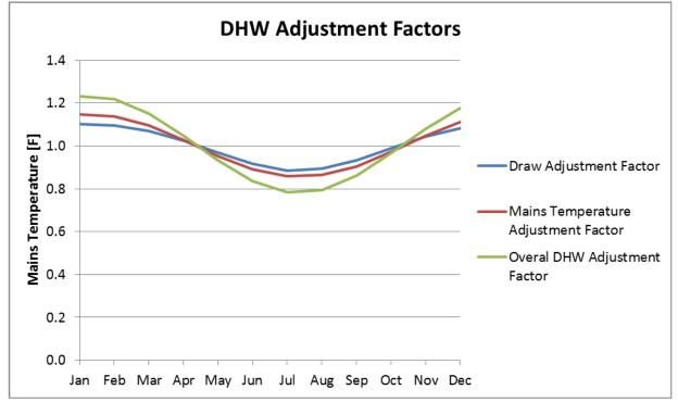
Figure 5-9. DHW Adjustment Factors, used to project DHW use for unmonitored months.
