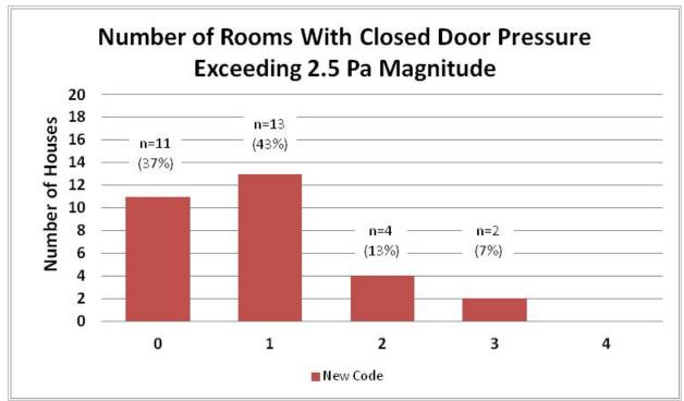
Figure 7-35. Distribution of homes having inadequate return air pathway for the new code group (n=30).
