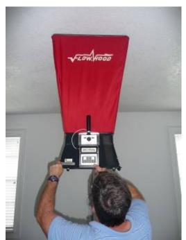
Figure 4-32. Airflows were also measured using a Flow Hood at return grills.
