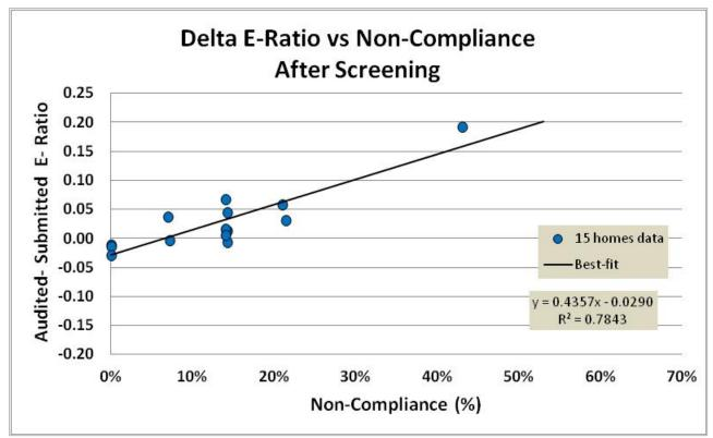
Figure 6-6. The difference between the audited and submitted e-ratios for 15 homes. Screening out the homes with over-compliance results in strong correlation.
