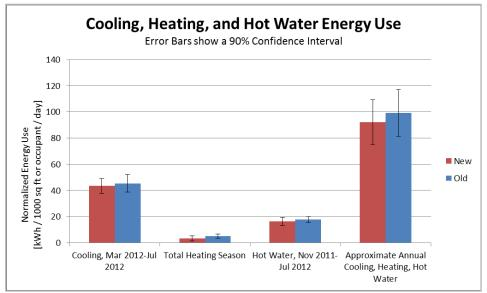
Figure 7-14. Overall Monitored Cooling, Heating, and Hot Water Energy Usage.
