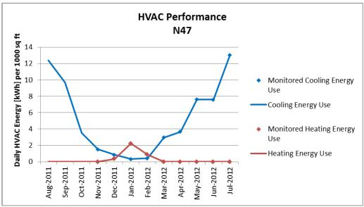
Figure 5-1. Chart of the final reported data for home 47. Note that this home only has monitored data from November 2011 to July 2012. Data before November 2011 has been projected (solid line) using one of the two methods described later in this report.
