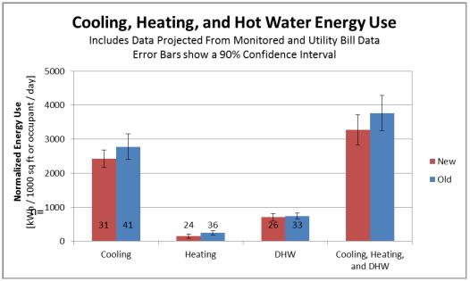
Figure 7-16. Overall Cooling, Heating, and Hot Water Energy Usage, Utilizing Monitored and Utility Bill Data Projections.
