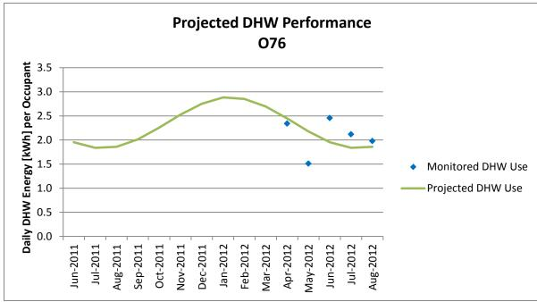
Figure A-207 Projected DHW Performance, O76
