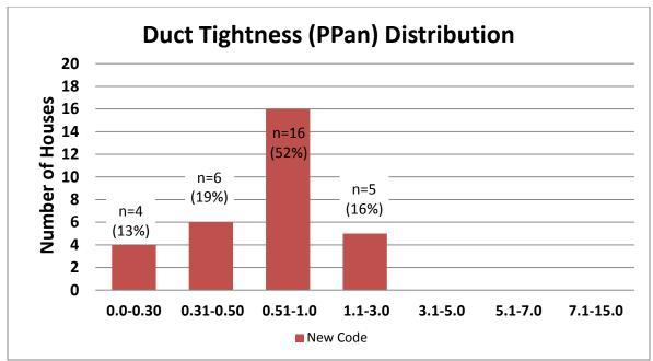
Figure 7-33. Duct leakage distribution for the new code group (n=31).
