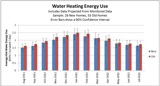
Figure 7-12. Hot Water Results Utilizing Monitored Data Projections.
