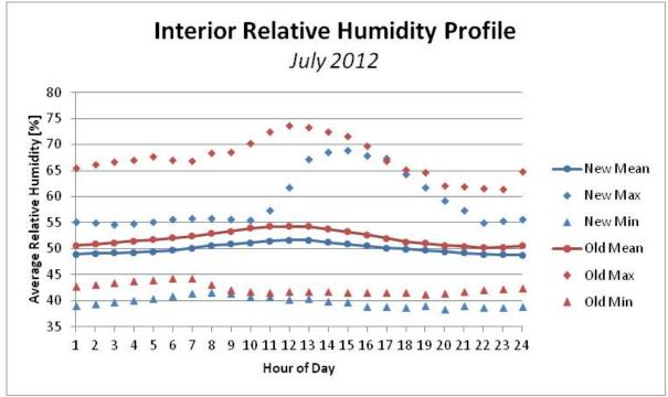
Figure B-24 Interior Relative Humidity Profile, July 2012
