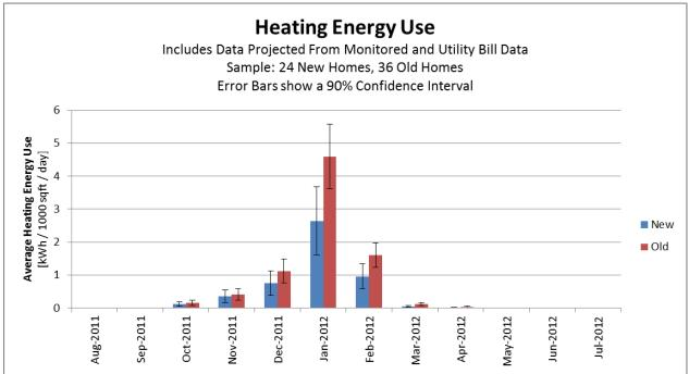
Figure ES-2. Monthly Heating Energy Use Results, Utilizing Monitored and Utility Bill Data Projections.
