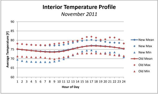
Figure 7-22. Interior Temperature Profile, November 2011
