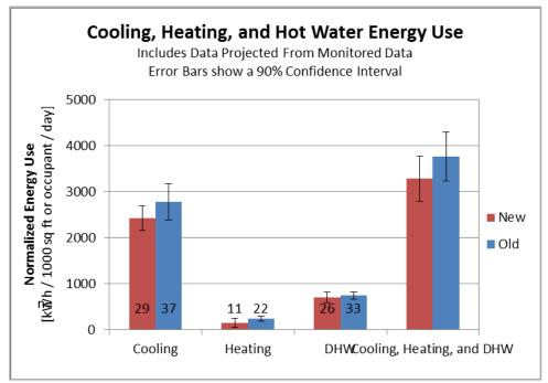
Figure 7-15. Overall Cooling, Heating, and Hot Water Energy Usage, Utilizing Monitored Data Projections.
