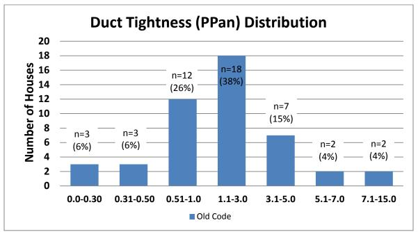
Figure 7-32. Duct leakage distribution for the old code group (n=47). (% may not add up to 100% due to rounding).
