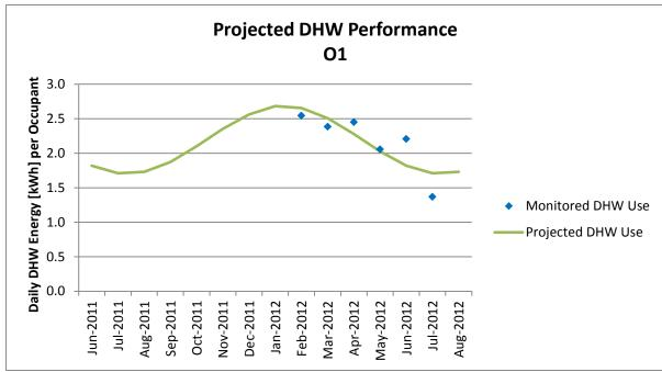
Figure A-95 Projected DHW Performance, O1
