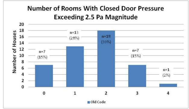
Figure 7-34. Distribution of homes having inadequate return air pathway for the old code group (n=46). (% may not add up to 100% due to rounding).
