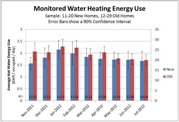
Figure 7-11. Monitored Hot Water Energy Use, Nov 2011-July 2012.
