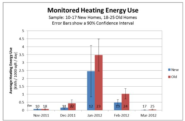
Figure 7-1. Monitored Heating Energy Use, Comparing New and Old Code Homes. Sample size is shown as a label at the base of each column.
