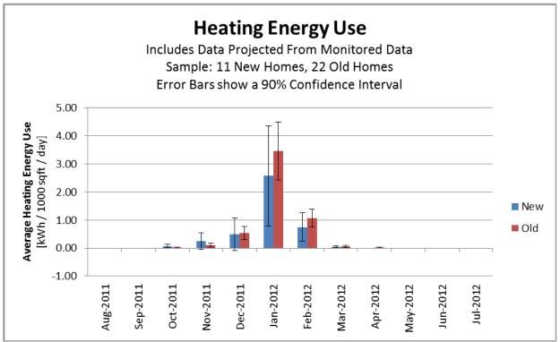
Figure 7-2. Heating Energy Use by Month, Utilizing Monitored Data Projections.
