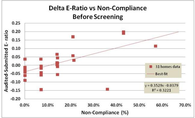
Figure 6-5. The difference between the audited and submitted e-ratios for 31 homes. Many of these homes have varying amounts of over-compliance as well as non-compliance.
