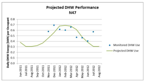
Figure 5-10. DHW performance, projected using the overall DHW adjustment factor.
