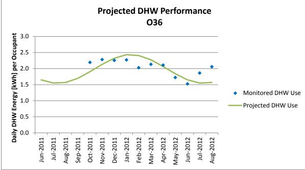
Figure A-152 Projected DHW Performance, O36
