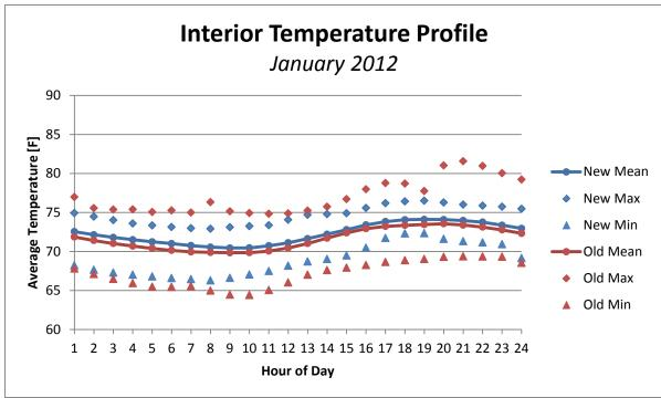
Figure B-11 Interior Temperature Profile, January 2012
