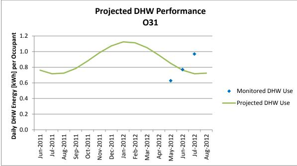
Figure A-142 Projected DHW Performance, O31
