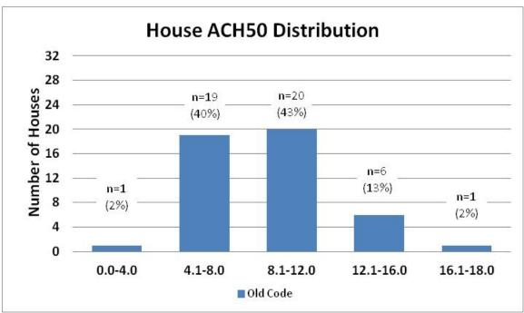
Figure 7-30. Normalized house leakage distribution for the old code group (n=47).
