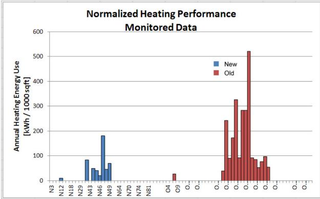
Figure 7-4. Monitored heating performance for each home, as calculated for November 2011 to Mar 2012.
