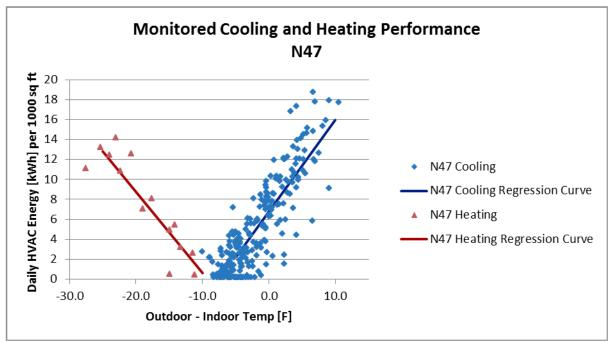
Figure 5-2. Chart showing the correlation between HVAC energy and the difference between indoor and outdoor temperatures. The regression curves are used to predict energy use values for missing months.
