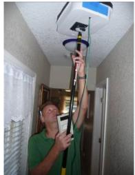
Figure 4-29. The pressure pan duct leakage test is used to indicate presence of significant air leakage near the supply and return grill measurements.
