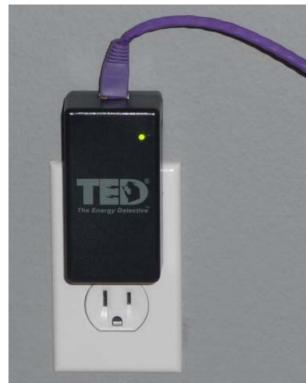
Figure 4-1. A TED energy data logger (gateway). The unit collects and stores data which can be accessed by internet using an ethernet connection. Current and voltage sensors called MTUs are located inside the electric service panel.
