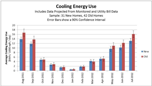
Figure ES-1. Monthly Cooling Energy Use Results, Utilizing Monitored and Utility Bill Data Projections.
