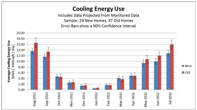
Figure 7-7. Cooling Energy Use by Month, Utilizing Monitored Data Projections.
