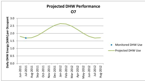
Figure A-105 Projected DHW Performance, O7
