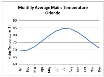
Figure 5-8. Water Mains Temperatures for Orlando Sanford Airport. These mains temperatures are used for all homes in the study because the differences between locations in Central Florida are small.
