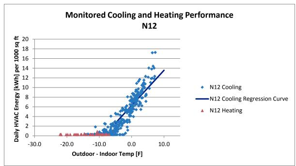
Figure A-13 Monitored Cooling and Heating Performance, N12
