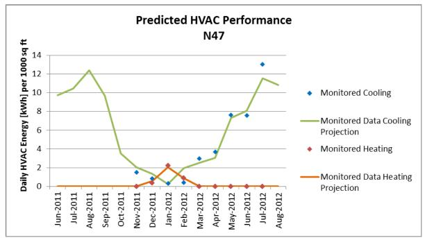
Figure 5-4. HVAC performance projected using a regression between monitored energy and the difference between indoor and outdoor temperatures.
