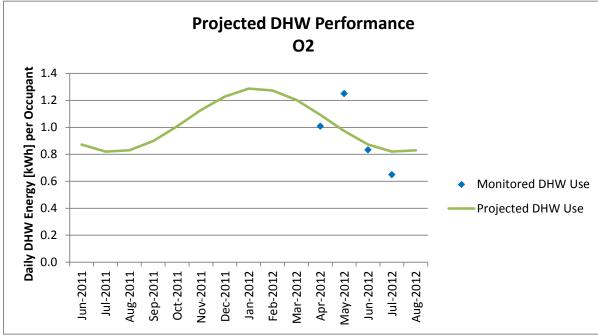
Figure A-98 Projected DHW Performance, O2
