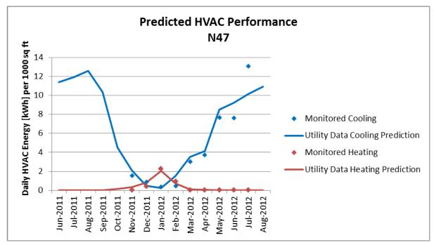
Figure 5-7. HVAC performance as predicted by utility bill analysis, after being scaled from a comparison between monitored data and predicted data.
