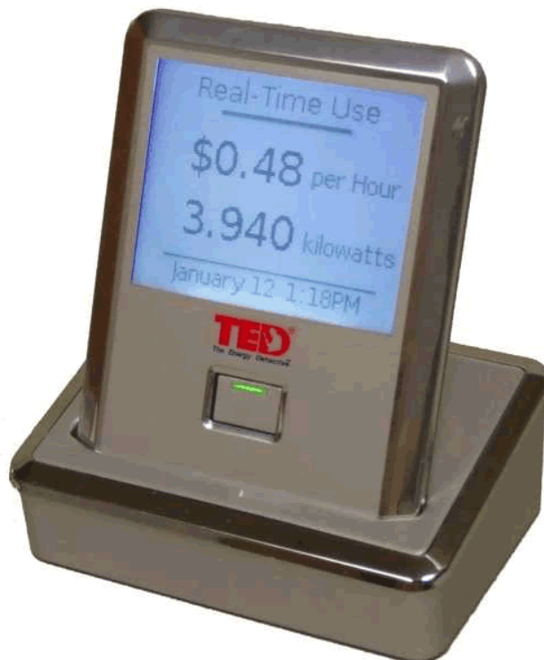
Figure 12. TED 5000 desktop display showing the house with an electrical demand of 3.940 kW
