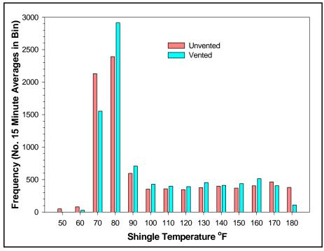
Figure 14. This histogram shows the comparative shingle temperature frequency distributions for the two test cells over the summer of 2000 with temperature bins of  $10^{\circ}F$ .
