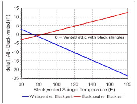
Figure 19. Plot of regression lines between white and black shingles over the temperature of the black shingle reference case.
