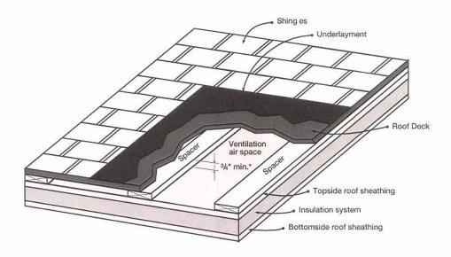
Figure C: Complete roofing assembly including spacers for ventilation
