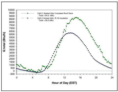
Figure 6. Estimated combined impact of duct heat gain, air leakage from the attic to conditioned space and ceiling het flux on space cooling needs on an average summer day in a  $2,000 \, \text{ft}^2$  home.
