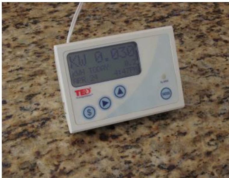
Figure 13. Installed TED energy feedback display.
