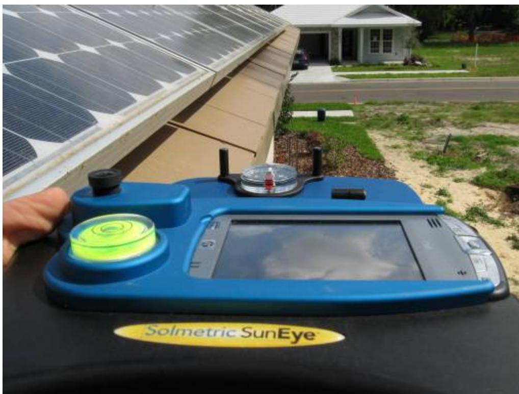
Figure 14. Evaluation of site shading using Solmetric Sun Eye.
